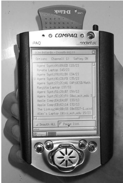
Figure 4: iPAQ H3600 with Dlink DWL-650 card, running Swat attack testing tool. Individual clients and AP's are identified either using MAC address or by passively monitoring the channel and extracting destination IP addresses and DNS names.
