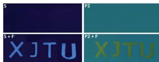
Fig. 7 The 5 and P2-based film sensors for fluoride anions under UV irradiation ( \lambda_{\text{ex}} = 365 \text{ nm} ).
