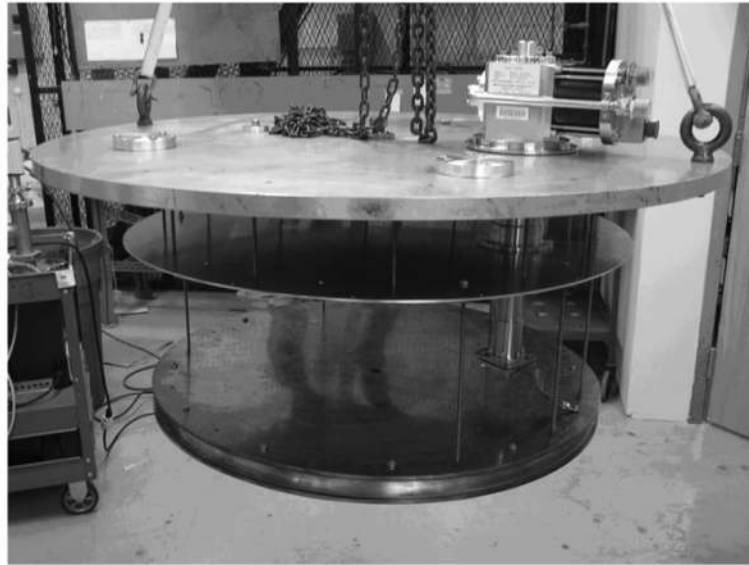
Fig. 7. Experimental setup for a single, conductively cooled, coil.
