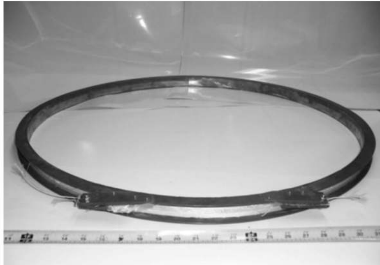
Fig. 9. Pre-heat treatment, single 770 mm ID coil wound with 400 m of unreacted multifilamentary \text{MgB}_2 conductor.
