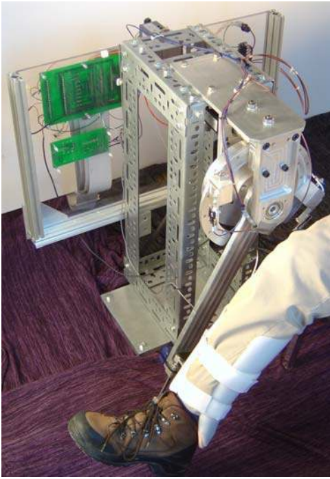
Fig. 3. 1-DOF exoskeleton for assisting knee-joint motion.
