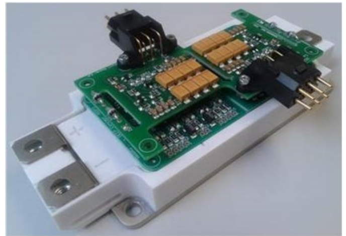
(a) Power module (with close control board)
