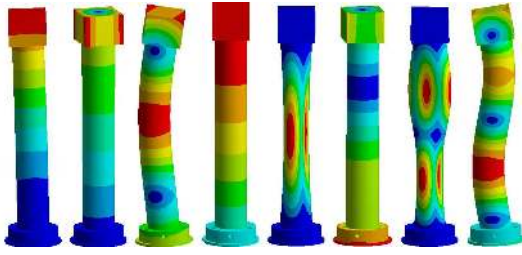
Fig. 3. ANSYS simulated mode shapes of the scanner (without sample mass). The casing of the scanner is hidden in order to display the mode shapes clearly. From the left, first bending mode: 658.4Hz; first torsional mode: 4.06kHz; second bending mode: 4.65kHz; first longitudinal extension mode: 5.76kHz; first circumferential mode: 9.25kHz; second torsional mode: 10.51kHz; second circumferential mode: 10.77kHz; third bending mode: 10.9kHz.
