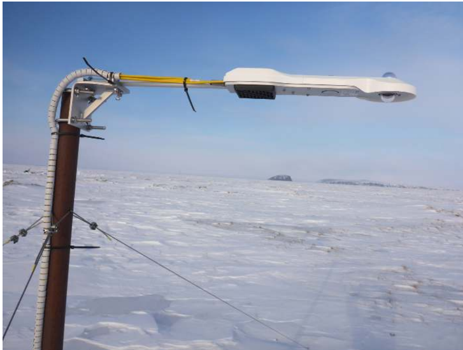
Figure B3. Kipp & Zonen CNR4 radiation sensor (including CNF4 ventilation unit) for measuring incoming and outgoing shortwave and longwave radiation installed on 22 August 2014.
