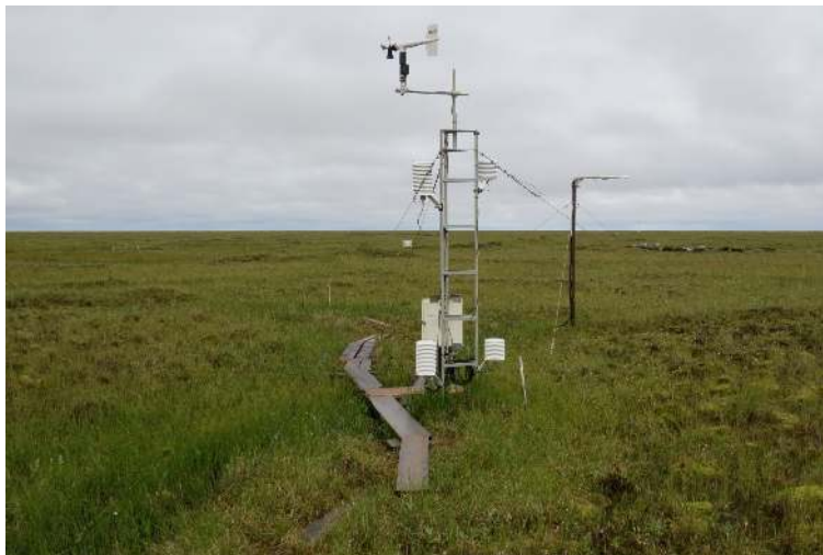
Figure B1. Samoylov meteorological station setup, August 2002–present ( 72.37001^{\circ} N, 126.48106^{\circ} E). Photo taken in August 2015. The two long radiation shields (left side of tower) at heights of 0.5 and 2 m house the combined temperature and relative humidity probes (two Vaisala HMP155A sensors were installed on 17 September 2017) and the two shorter shields (right side of tower) at the same heights contain Campbell Scientific PT100 sensors (installed on 22 August 2013) to measure air temperature only. The data logger (Campbell Scientific CR1000, installed on 30 June 2009), multiplexer (Campbell Scientific AM16/32A, installed on 27 July 2010) and barometric pressure sensor (Vaisala PTP110, installed on 22 August 2014) are located in the white box at the back of the tower. The wind monitor and radiation sensor are shown in the figures below (Figs. B2 and B3).
