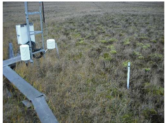
Figure D3. Installation for water-level measurements using a permeable ground water measurement tube with a Schlumberger Mini-Diver.
