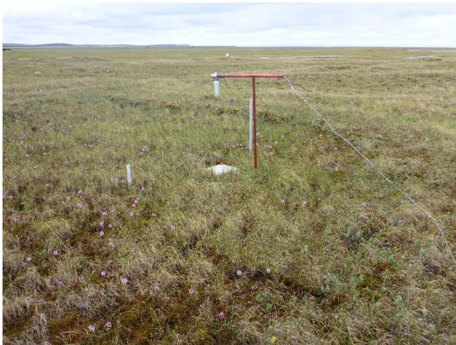
Figure B4. Campbell Scientific SR50 snow depth sensor, installed on 24 August 2002. An aluminum plate was installed on the ground surface beneath the sensor beam on 17 July 2015.
