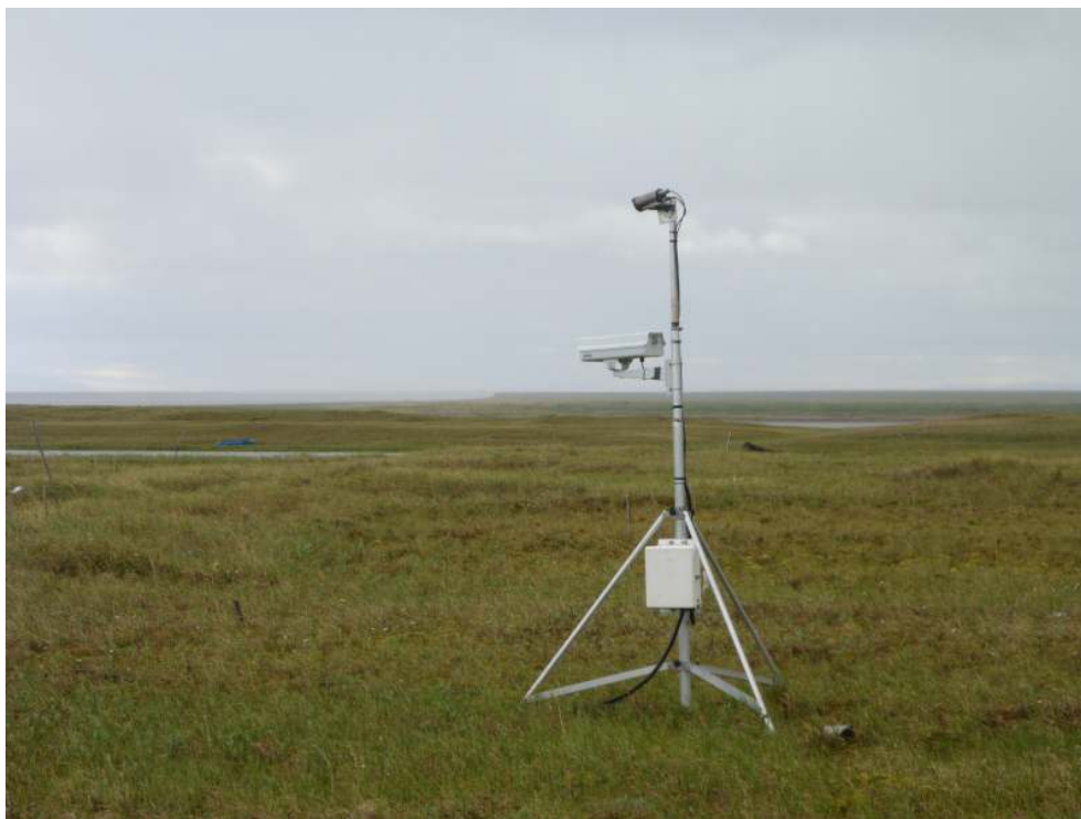
Figure B5. Cameras for time-lapse photography of snow cover and land surface pointing towards the polygon field: a Campbell Scientific CC5MPX at the top (since 4 August 2015) and a Campbell Scientific CC640 below (since 1 September 2006). Photo taken in 2016.
