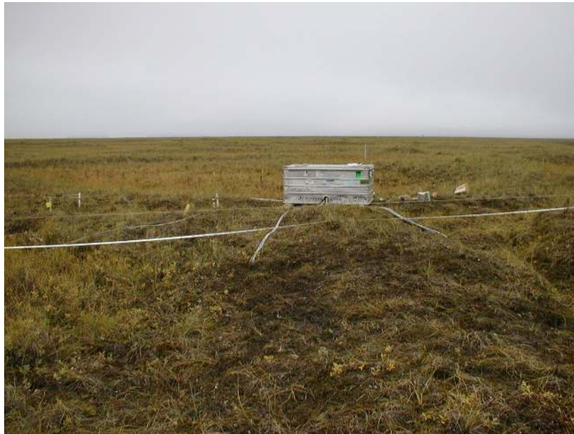
Figure B10. Research site after instrument installation in soil pits and subsequent refilling, August 2002. Cable strings indicate locations of centre, slope, and rim profiles.
