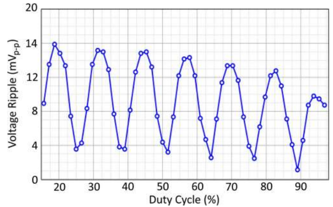
Fig. 16. Output voltage ripple of an IVR with Type 2 silicon interposer operating at 100 MHz switching frequency.
