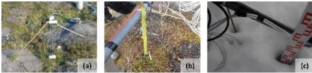
Figure C5. (a) Vertically installed time-domain reflectometry (TDR) air–snow TDR probe (50 cm length) above the ground surface during summer at the Bayelva climate station (1999). During winter (fully snow covered), the dielectric number of snow is recorded. (b) PT100 temperature sensors in air (summer) at 4 and 20 cm above ground surface. (c) PT100 temperature sensors in snow (winter) with air gaps around cables and sticks; the TDR probe is completely covered with snow and not visible from the surface.
