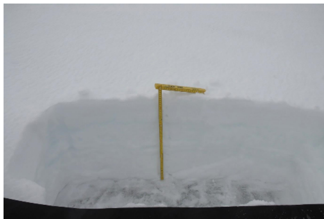
Figure E3. Snow pit, 10 May 2016. The basal ice layer is visible at the bottom of the snow layer. Two profiles were measured: one to the left and one to the right from the yellow meter stick (profile data named left and right in Table E1). Further data on temperatures, dielectric numbers and stratigraphy can be found in Table E1.
