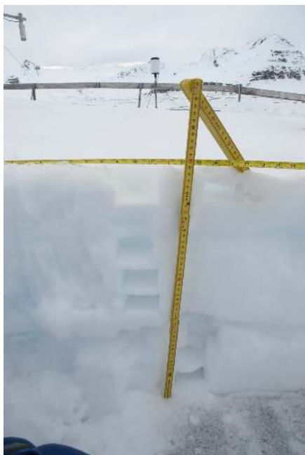
Figure E2. Snow profile taken on 9 May 2016, inside the Bayelva fenced area. The pockets/holes are the result of snow removal using a snow density cutter ( 100\text{ cm}^3 ). Snow depth is 47 cm above a basal ice layer at the point of measurement but ranges between 47 and 49 cm. Measurements were taken to the left of the yellow folding rule (left and right profiles in Table E1). Ice layers are present 24–28, 43–47 and 55–56 cm above the basal ice layer, which is 15 cm thick. Further data on temperatures, dielectric numbers and stratigraphy can be found in Table E1.
