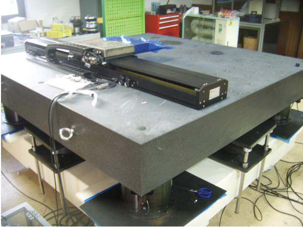
FIGURE 4: An air mount with EM actuators.
