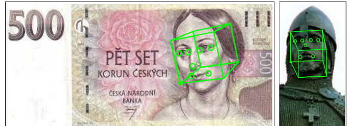
Fig. 1. The proposed method jointly estimates the position of seven facial landmarks in the image and the head pose (position and orientation) with respect to the camera frame. The landmarks are shown as circles and the pose is visualized by projecting a virtual 3D cube around the head into the image. The method is robust, the classifier generalizes even to images of an artistic engraving or a bronze statue.
