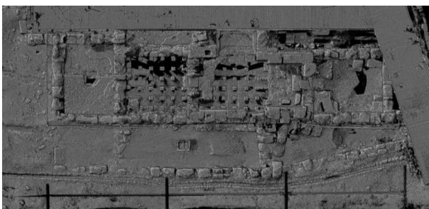
Figure 3. Top view of the 3D Model of the Roman baths area, range based reconstruction.
