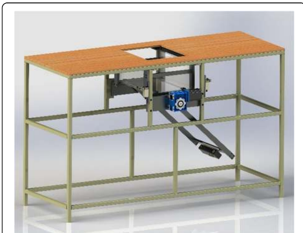
Fig. 1 The self-developed foot shape 3D scanning system based on Kinect 2
