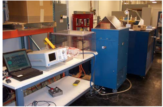
Fig. 10. Inductive load test set-up.
