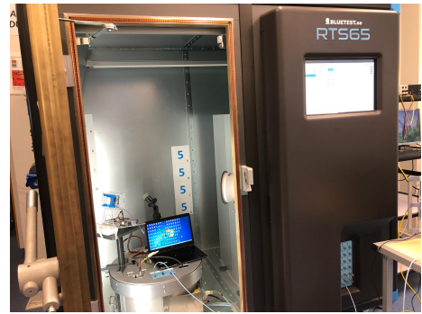
Fig. 3. Reverberation chamber OTA measurement setup using Bluetest RTS65. All elements within chamber, including PC, were taking into account during calibration.
