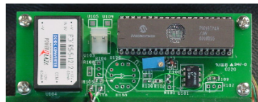
(b) The PID controller implemented with a PIC RISC microcontroller
