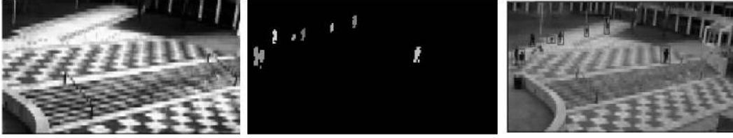
Fig. 2. Background mean image, blob segmentation image, and input image with blob bounding boxes.
