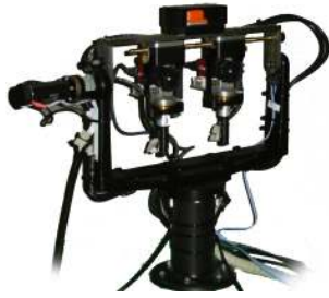
Figure 1. View of the current version of the Integrated Multimodal Perception Experimental Platform (IMPEP). The active perception head mounting hardware and motors were designed by the Perception on Purpose (POP - EC project number FP6-IST-2004-027268) team of the ISR/FCT-UC, and the sensor systems mounted at the Mobile Robotics Laboratory of the same institute, within the scope of the Bayesian Approach to Cognitive Systems project (BACS - EC project number FP6-IST-027140).
