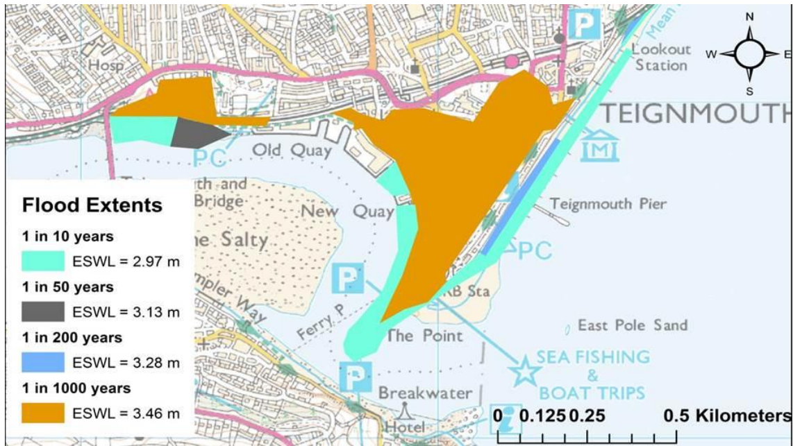
Figure 10: Network model flood extents for four extreme still water levels with the new 1 in 200 year estuarine tidal-flood defence
