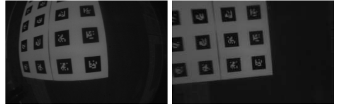
Fig. 6. Images from downward looking camera before and after undistortion.
