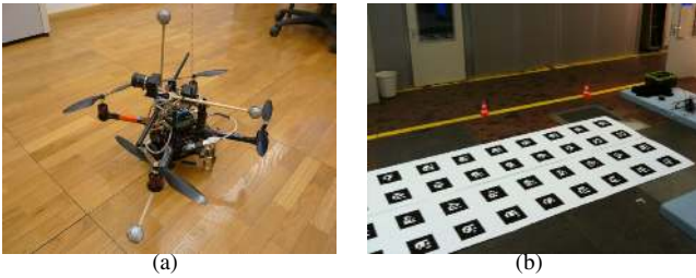
Fig. 1. (a) The “Pelican” quadrotor equipped with a forward looking camera, a downward looking camera, an IMU, and three reflective markers for the Vicon system. (b) Group of ARToolKitPlus markers placed in known location.
