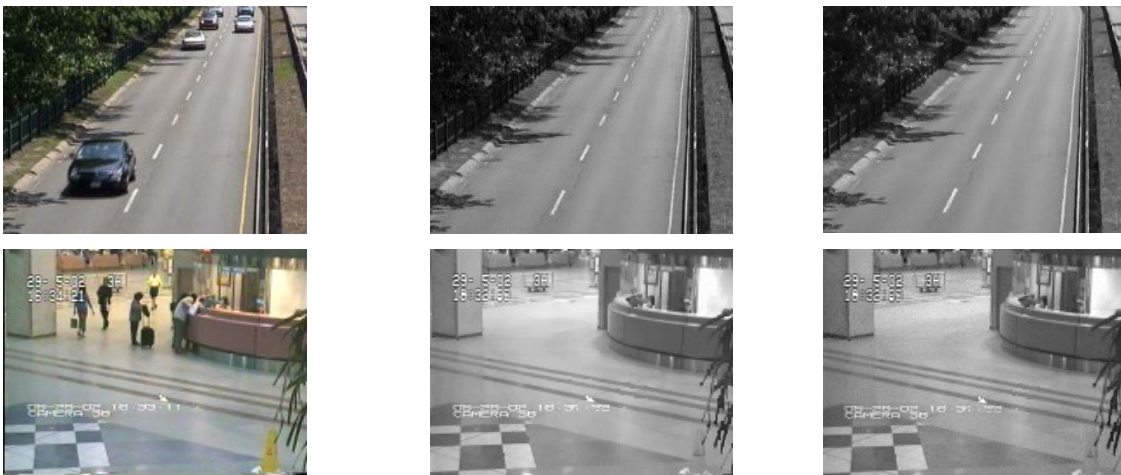
Fig. 4. Background images of “Highway” and “Airport” sequences, first column: an image of the sequence, second column: initial background model, third column: background model after 1000 frame.
