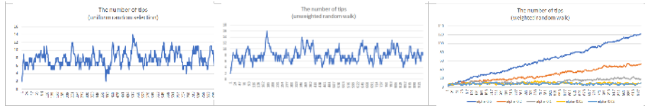
Fig. 6. Number of unconfirmed tips under (a) uniform random selection, (b) unweighted random walk, and (c) weighted random walk.
