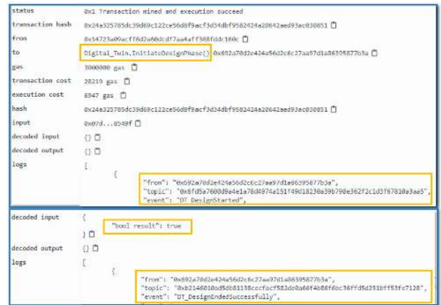
FIGURE 6. Logs presenting a successful beginning and end of the design phase by the design manager.
