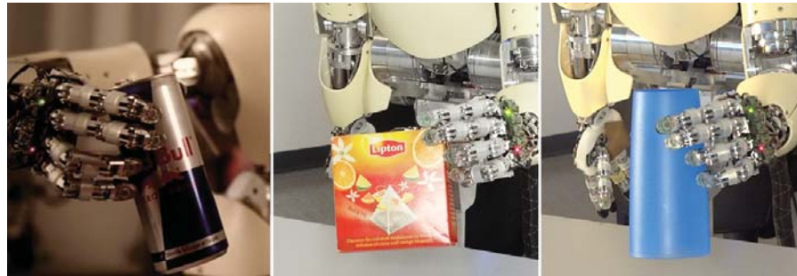
FIGURE 10.6 Grasping a variety of objects successfully, such as, tin cans, plastic cups and tea boxes. The module works for both the right and left hand.
