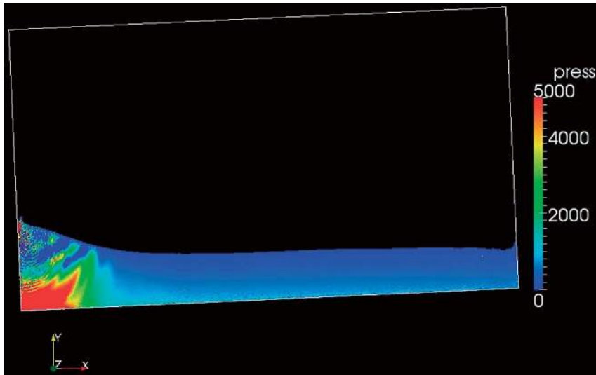
Fig. 10. Pressure field [Pa] at the pressure peak instant.
