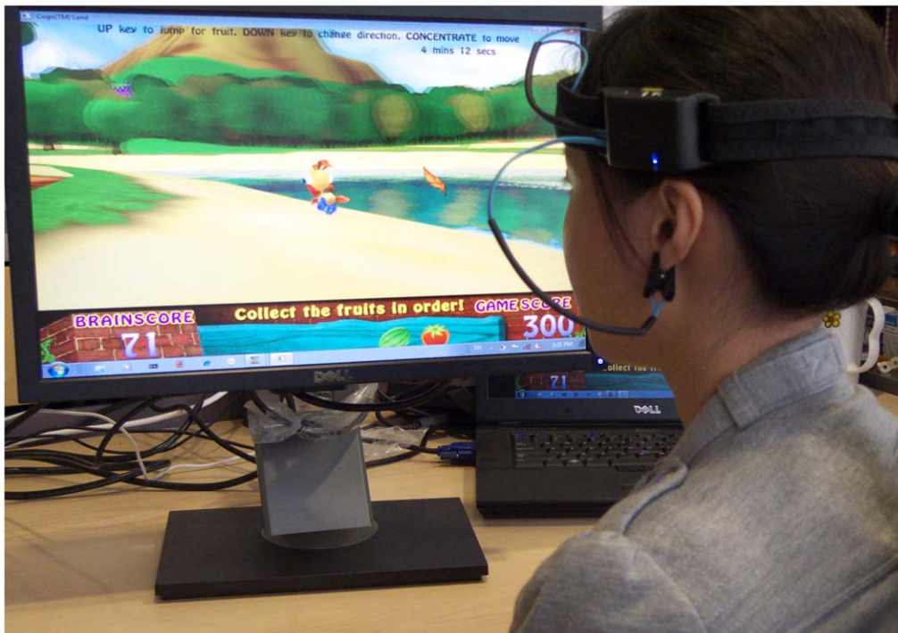
Figure 2. A model engaged in intervention with the Brain-Computer Interface (BCI) attention training game system. doi:10.1371/journal.pone.0046692.g002
