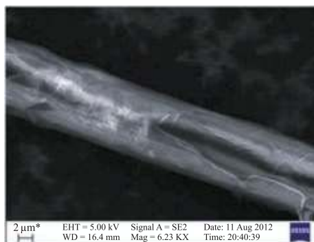
Figure 10: Scanning electron microscopic image of GO coated etched FBG. 48
