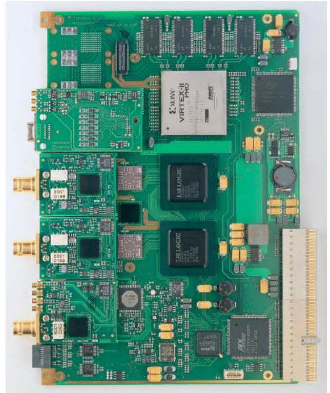
Fig. 1. Board of AC240, the hardware of the FFT spectrometer. On the left, from top to bottom, are the system control interfaces, two analog inputs for the signal at intermediate frequency (SMA connectors will be used in the final version), and an input for a trigger or a clock. The FPGA processing unit is visible in the top center, the PCI bus for data output at the bottom right.
