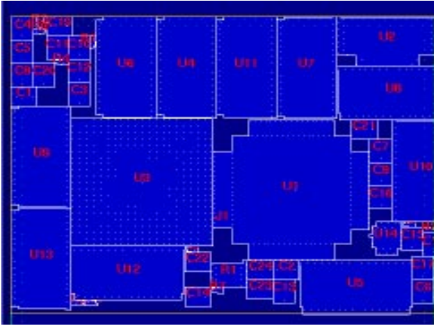
Fig. 12. Sample placement of design 1051703 using an area weight of 1, an interconnect weight of 1, and 6 inner loop iterations.
