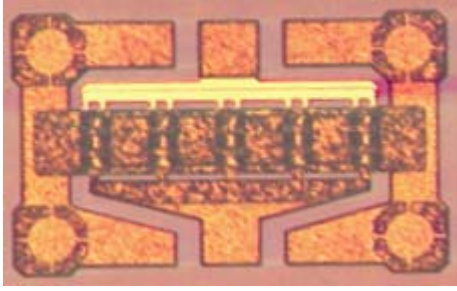
Fig. 2: Microphotograph of the GaN HEMT device.
