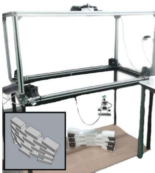
Fig. 1 The layout of the SPIDERobot. The example of an architectural project is depicted in the left–bottom side
