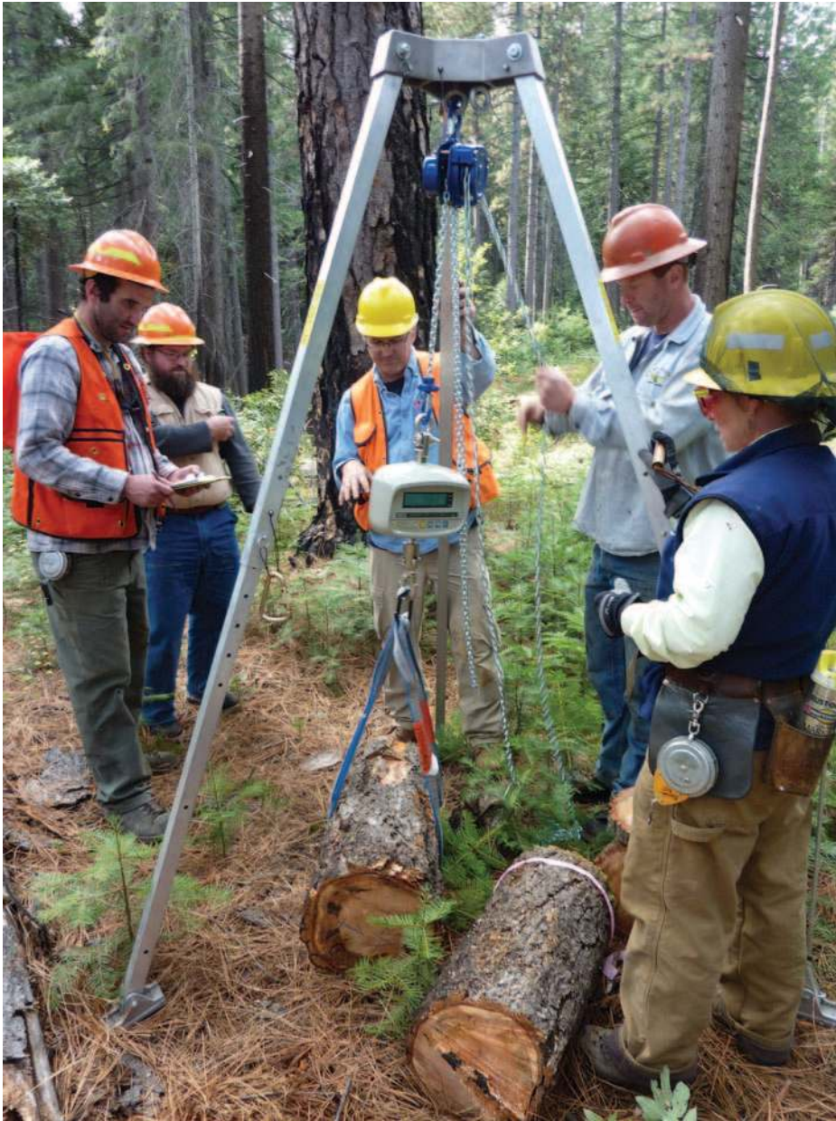
Figure 1. USDA Forest Service measurement specialists weighing stem sections at a Check-Cruiser workshop on the Tahoe National Forest in California, October 2014. Photo by Ruth Rieper.
