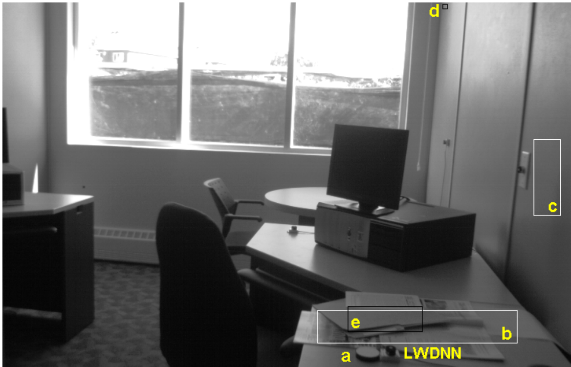
Figure 4 View of Room B from the perspective of the camera used for control. Superimposed are the points/areas used for control criteria in the early trials. (LWDNN) is the desktop illuminance sensor; (a) is the reflectance standard; (b) is the desk area; (c) is the wall area behind the computer from the occupant perspective; (d) is the wall area near the window; (e) is an alternate desk area used for a ratio with area (d). Note, when the camera was used to control the motorized blind, the field of view was changed slightly to incorporate the upper part of the window
