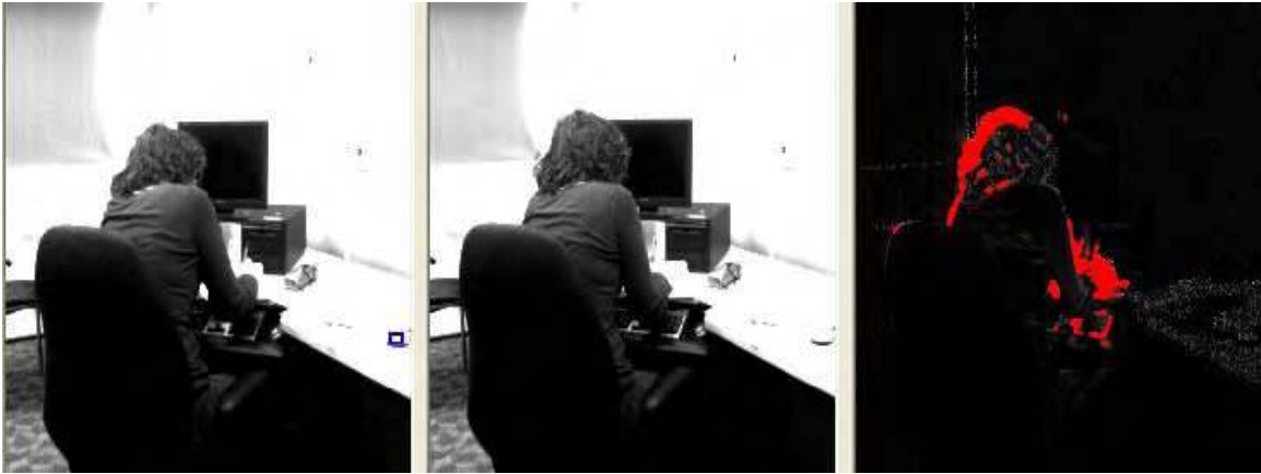
Figure 12 An example of the image subtraction technique for occupancy sensing. The images to the left and in the middle were taken one minute apart. The area of the reflectance standard used for image calibration is shown by the blue square on the left. To the right is the result of subtracting the two images. Pixels where the difference was greater than 5 \text{ cd/m}^2 are shown in red. Even small changes in body/object positions are clearly captured
