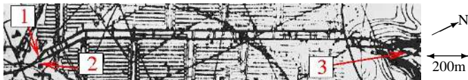
Fig. 6. The prior map of Mathies, with the three portals labeled. The corridors of interest run horizontally from left to right. Note the inaccuracy in the map on the right side (the corridors are misaligned). The image represents approximately 1200 meters from left to right.
