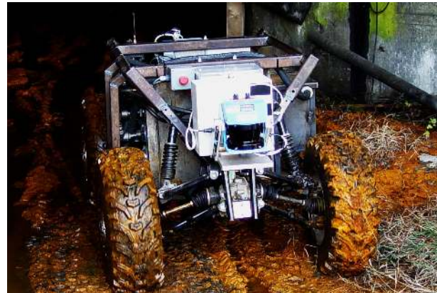
Fig. 1. Groundhog: a rugged platform designed to traverse the rough, unpredictable terrain of mine corridors, able to overcome obstacles such as fallen roof timbers, partial sidewall or roof collapses, rail tracks and deep mud. Shown here at the north portal to the Mathies mine.
