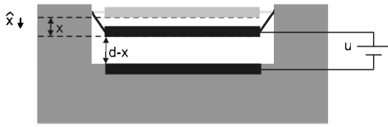
Figure 1. Schematic drawing of a parallel plate capacitor with one movable plate.
