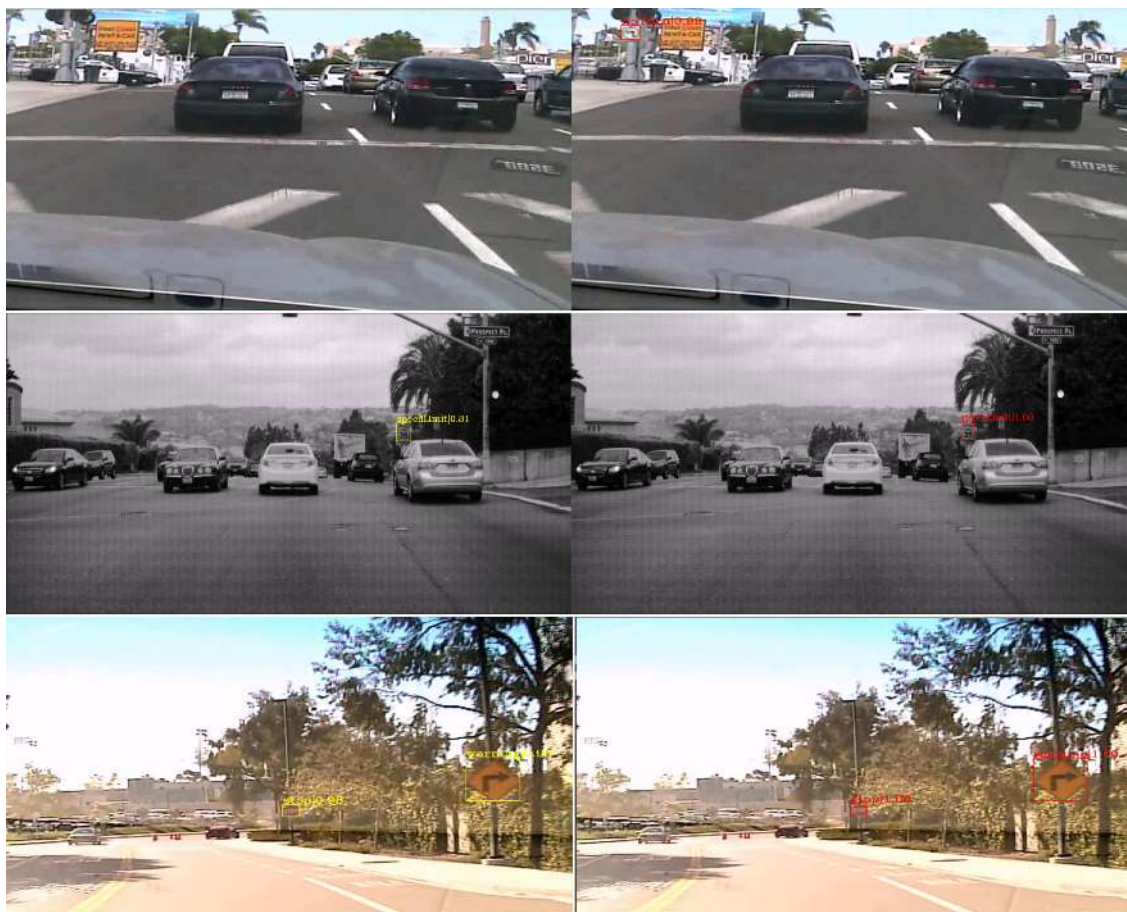
FIGURE 11. Traffic sign detection results in Lisa dataset. The detection results of cascaded R-CNN network are shown on the left, and the results of network with our proposed method are shown on the right. Especially, the target of images in the first row is undetected using the cascaded R-CNN network on the left while it is detected using our proposed method on the right.
