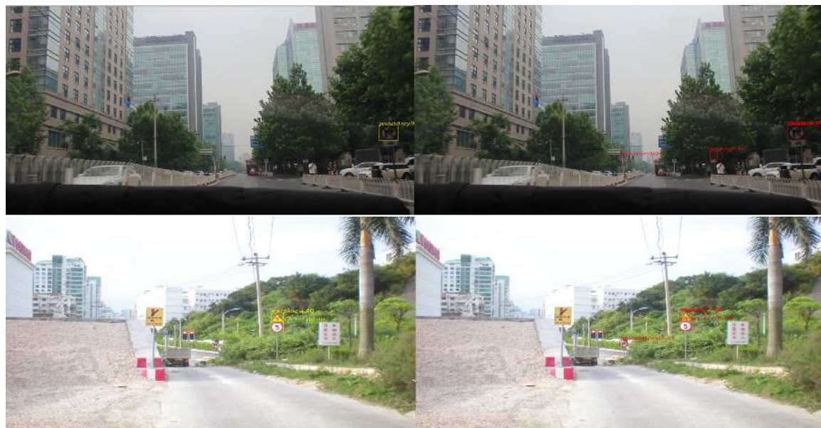
FIGURE 13. Traffic sign detection results in CCTSDB. The detection results of cascaded R-CNN network are shown on the left, and the results of network with our proposed method are shown on the right. The targets of images using the cascaded R-CNN network on the left are undetected and false detected while they are detected on the right.
