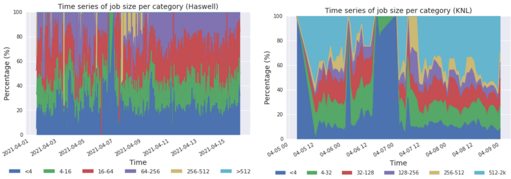
Fig. 1. Area plots for the size of jobs nodes are assigned to, for Haswell (left) and KNL (right) nodes.
