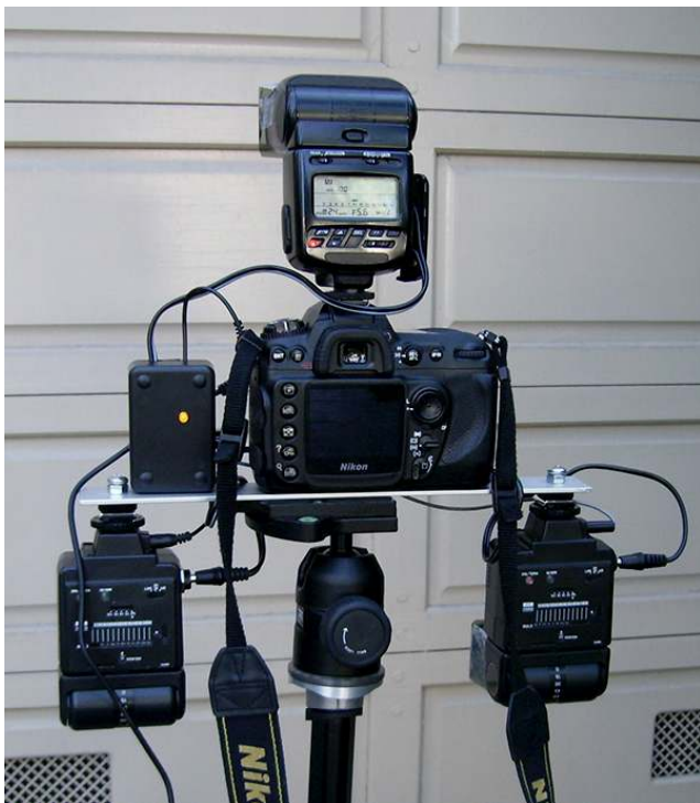
Figure 2. Three-flash capture system mounted on a tripod with a digital SLR camera.
