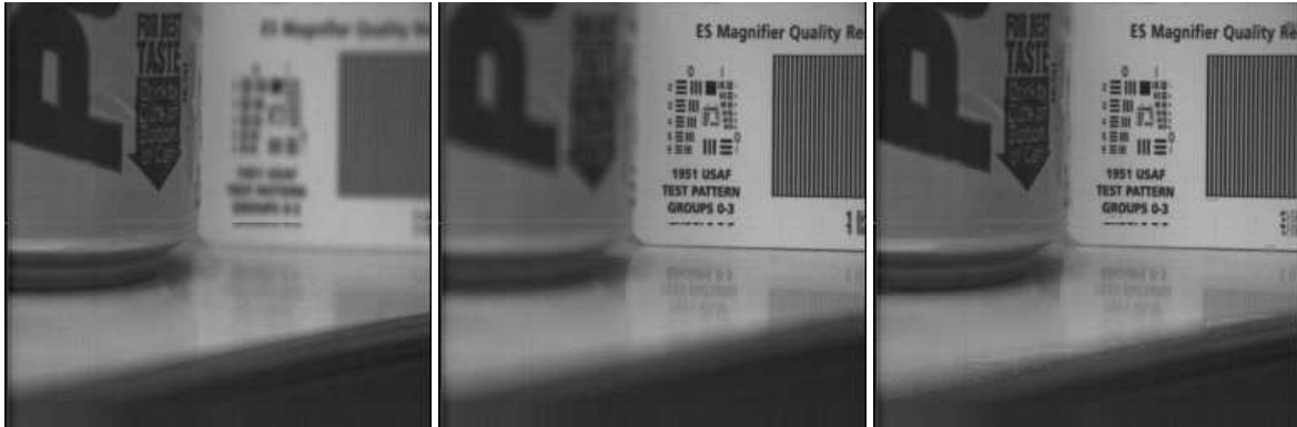
(a). Image 1 (focus on left) (b). Image 2 (focus on right) (c). Fused image (all focus) *
