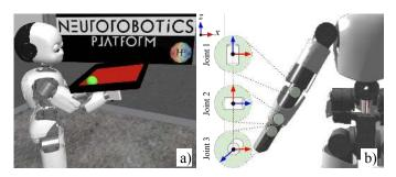
Fig. 1: Robotic plant: **a**) the humanoid iCub holding the table-ball system in the Neurorobotics Platform; **b**) the three controlled wrist joints: **1** pronosupination, **2** yaw, **3** pitch.
