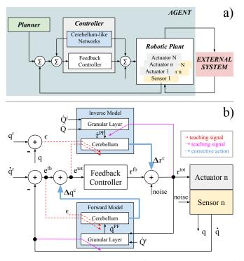
Fig. 2: Control architecture scheme for N actuated joints: **a**) main components communication, and **b**) controller block.
