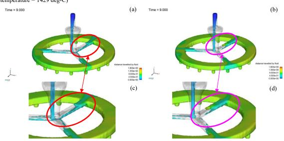
Fig. 7 Contour of distance traveled by the molten metal on 9s at (a) 1329 deg-C, (b) 1529 deg-C of the pouring temperature, (c) a close-up view of 1329 deg-C, and (d) a close-up view of 1529 deg-C
