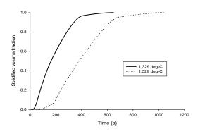
Fig. 8 Comparison of the solidified volume fraction of each pouring temperature through the solidification process
