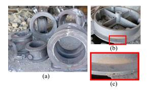
Fig. 1 Plumbing joints produced in the plumbing manufacturing process (Thailand); (a) examples of plumbing parts, (b) an example of defected part, and (c) a close-up view of the porosity occurrence
