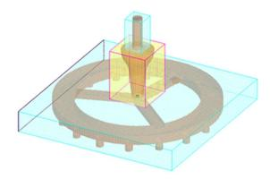
Fig. 3 The multi-block meshes of the plumbing component (the mould mesh is not displayed).
