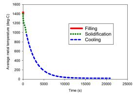
Fig. 6 Average temperature occurrence during the filling, solidification, & cooling stages (pouring temperature = 1429 deg-C)
