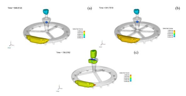
Fig. 9 Defect net volume on 1329 deg-C of the case (a) 3 branches runners, (b) 6 branches runners, and (c) 3 branches15-degree inclined runners
