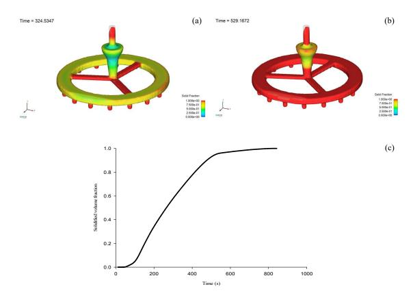
Fig. 5 The solidification of the plumbing component at (a) 0.6 solid fraction, (b) 0.9 solid fraction, and (c) solidified volume fraction through the solidification process
