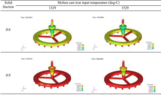
Table 3 The solidification of the plumbing component at 0.6 and 0.9 solid fraction comparing between the cases 1329 deg-C and 1529 deg-C of pouring temperatures.
