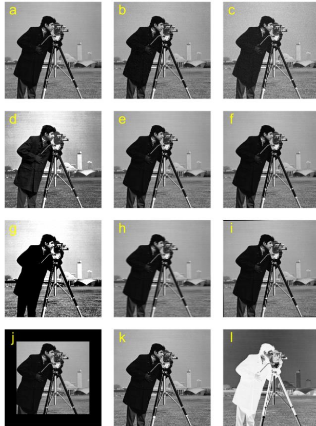
Fig. 5 Watermarked image under different attacks. (a) JPEG compression (70%), (b) Salt & pepper noise (10%), (c) Gaussian noise (0,0.01), (d)Histogram Equalization, (e) Median filter [3×3], (f) Low-pass filter [5×5], (g) Gamma correction (0.6°) (h) Motion blur (45°) (i) Rotation (1°), (j) Cropping (25%) (k) Sharpening (l) Complement.
