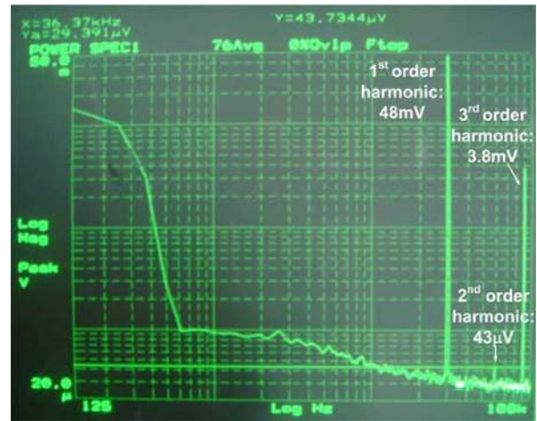
Fig. 22. Measured chopper ripple with the RRL “off”.
