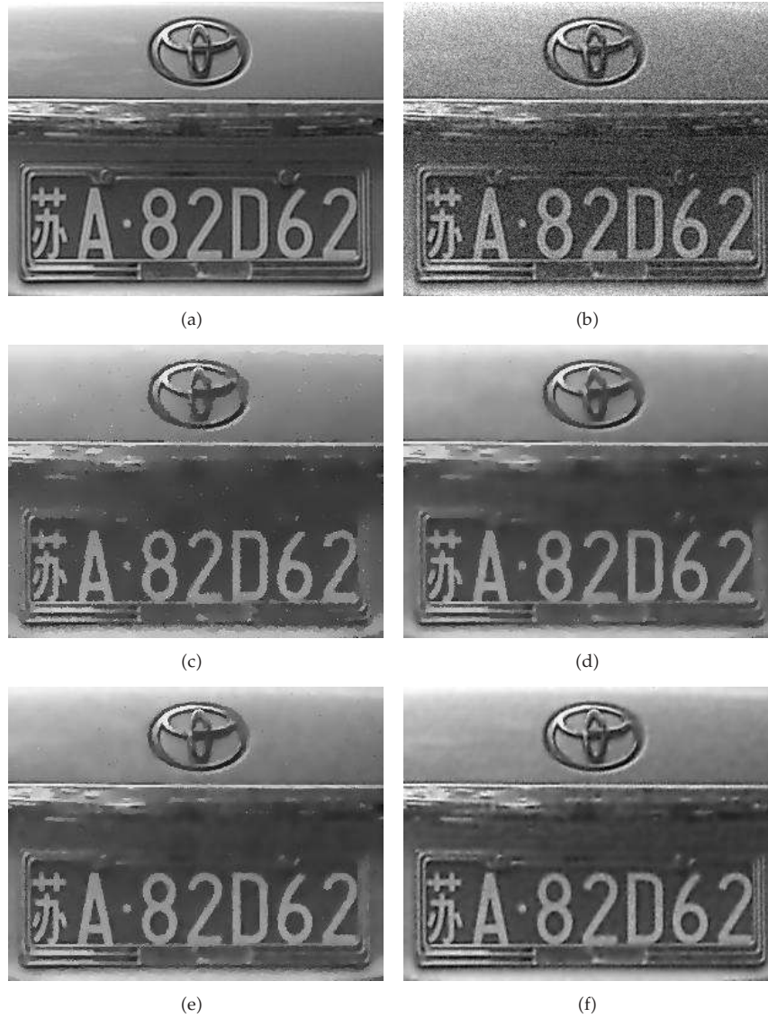
Figure 3: Comparison of different methods on “License plate” image. (a) Original image. (b) Noisy image. (c) PM smodel with k = 10 . (d) TDE model with k = 10, \lambda = 40 . (e) ITDE model with k = 10, \lambda = 40, \sigma_1 = 0.1 . (f) Proposed fourth-order TDE with k = 1, a = 4, \lambda = 10 .
