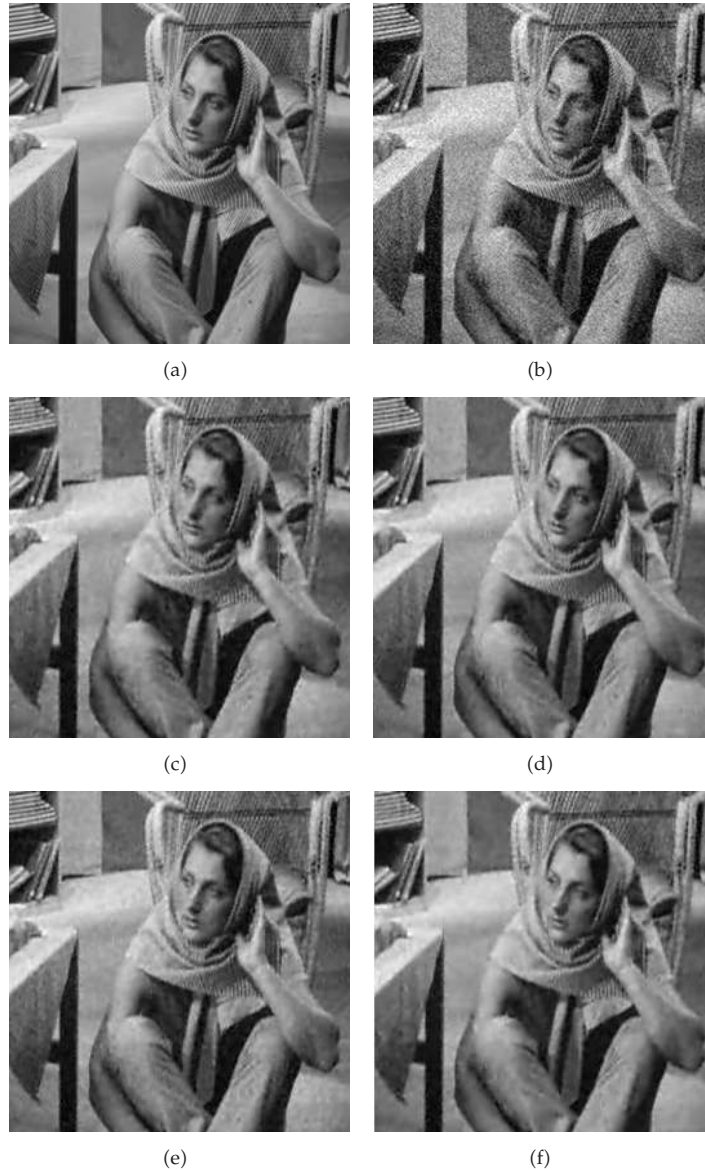
Figure 1: Comparison of different methods on “Barbara” image. (a) Original image. (b) Noised image. (c) Fourth-order TDE with \lambda = 1 . (d) Fourth-order TDE with \lambda = 40 . (e) Fourth-order TDE with \lambda = 70 . (f) Fourth-order TDE with \lambda = 100 .
