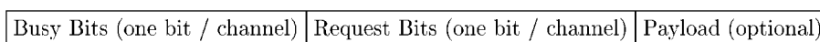
Fig. 10. The layout of a THORN-based token request packet. Each token packet contains one bit per channel for busy status and one bit per channel for the channel requests. The token packet also contains an optional payload for small, low latency messages.
