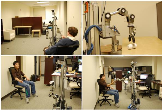
Fig. 7. Each row shows the user clicking a button and the robot selecting the appropriate behavior when the robot is in the Object_In_Gripper state. Top to bottom: Deliver_To_Table , Deliver_To_Person
