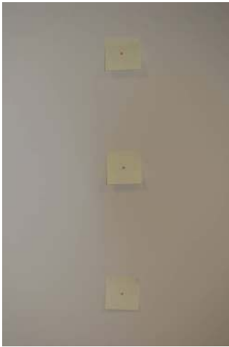
Fig. 9. Wall buttons that the robot is supposed to touch. Success in this task is defined as the robot touching the yellow square (7.7 cm) on which the red targeting dot was placed.
