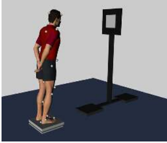
Fig. 1. Experimental device. Physical target moved by a linear motor, force plate and motion capture device.
