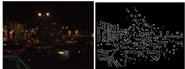
Figure 4: One image before and after canny edge detection. The original (left) is one we class unmemorable and the result after edge detection is that less than 10% of the image contains edges.
