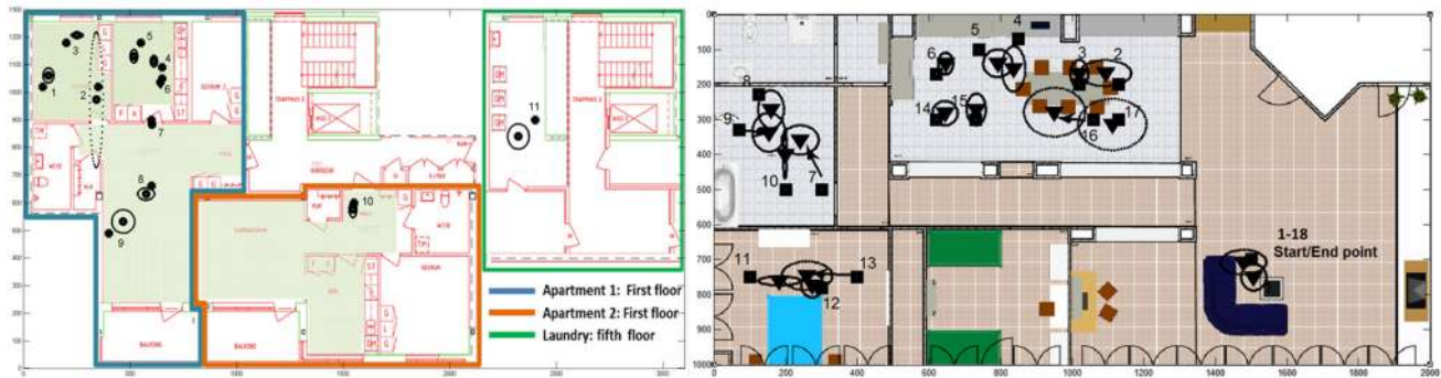
Fig. 6 Representation of the localization outputs from the ULM inside the Domocasa ( right map ) and the Angen ( left map ) sites. The black squares represents the actual user positions, while the estimated users
