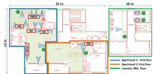
Fig. 3 The LNet and SNet setups in the Angen experimental site (Sweden). Specific markers represented the position of each environmental sensor and router device of the SNet. Red squares and colored circles represented respectively the presence sensors and the environmental sensors, while rings identify the Routers devoted to the multi hop communication between the sensors in the laundry at the fifth floor and the rest of the sensor network in the apartments at the first floor. The LNet devices are represented by blue cones that defines the position and orientation of the connected sectorial antennas. while for each anchor devoted to the user localization, a blue cone highlighted the position and orientation of the connected sectorial antenna. (Color figure online)
