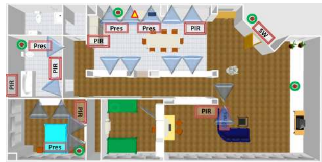
Fig. 2 The LNet and SNet setups in the Domocasa Lab experimental site (Italy). Specific markers represent the position of each wireless board connected to the LNet and the SNet. Red squares identify the presence sensors, colored circles the environmental sensors measuring temperature, light and humidity, a blue cone highlighted the position and orientation of the connected sectorial antenna for each anchor devoted to the user localization. (Color figure online)
