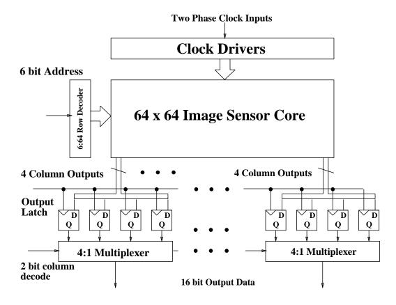
Figure 2: Figure 2: Image Sensor Chip Functional Block Diagram. TP-13.5: "A CMOS Area Image Sensor with Pixel-Level A/D Conversion", Boyd Fowler, Abbas El Gamal, and David X. D. Yang
