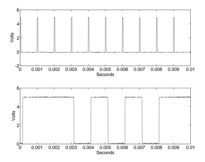
Figure 3: Figure 3: Single pixel Sigma-Delta modulator output from HP54601A. The top graph is **PHI2** versus time and the bottom graph is the pixel output waveform versus time. TP-13.5: "A CMOS Area Image Sensor with Pixel-Level A/D Conversion", Boyd Fowler, Abbas El Gamal, and David X. D. Yang
