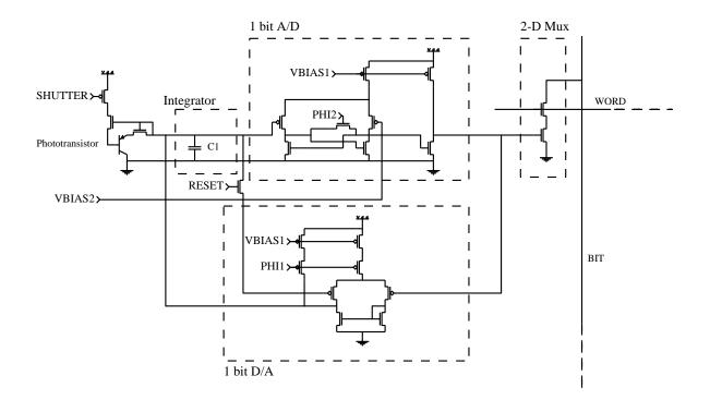
Figure 1: Figure 1: Pixel Schematic. TP-13.5: "A CMOS Area Image Sensor with Pixel-Level A/D Conversion", Boyd Fowler, Abbas El Gamal, and David X. D. Yang
