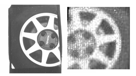
Figure 4: Figure 4: 300dpi scan of print from negative (left).  $64 \times 64$  image produced by sensor using 35mm negative contact exposure (right). TP-13.5: "A CMOS Area Image Sensor with Pixel-Level A/D Conversion", Boyd Fowler, Abbas El Gamal, and David X. D. Yang
